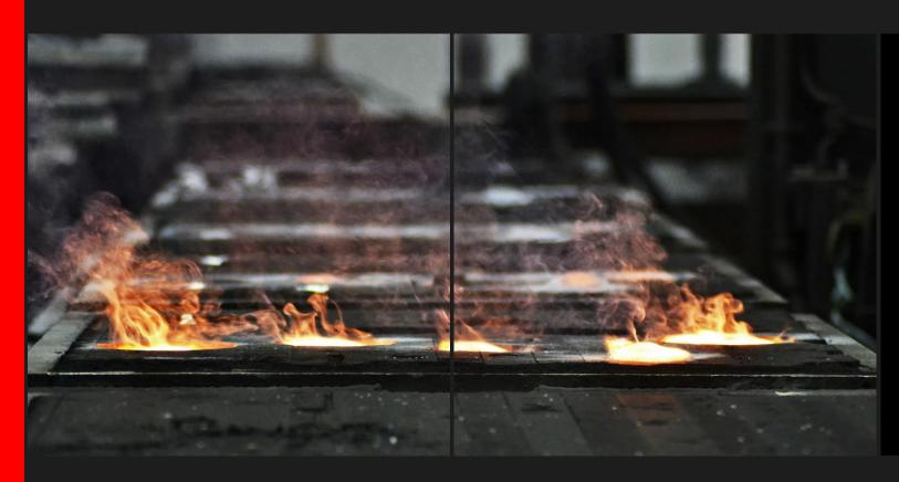
Automatic plant with 3 robots for GREEN SAND casting Prototypes and series Max. Dimension: 1000 X 800 Max. Weight: 150 kg
